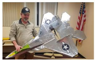
**2.** Ken K. scratch built this F22 using 1/2" blue foam. It sports a 100A speed controller and 6C 4500 LiPO. Nice Job.
