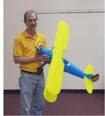
2. Mike has been keeping his PRUSA-I3 3D printer humming building this PT-17 Kaydet from 3D Lab-Print plans. He used PLA plastic for the majority of the build. His 47.9" wingspan plane weighs 5 1/2# and is powered with a Suppo 2826-? Motor.
