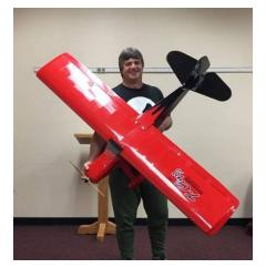
2. Gary brought this Sig T-Clips ARF. The 70" wingspan plane has a Turnigy L5055A-400 motor, 85A ESE and 5000mah 6c LiPO. Gary said it draws 44A w/ 15-8 prop.
